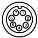
7 pins Binder 712 male connector pinout Solder termination view
